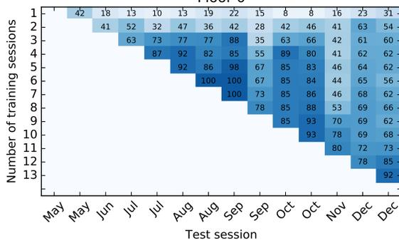
Fig. 4. CSI-based localization performance over time, with incremental training. Numbers in the cells are percents of correctly recognized fingerprints. Random-guess levels are 3% (Offices) and 8% (Campus).
