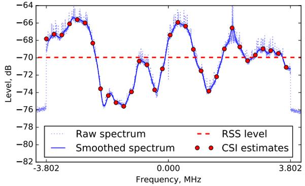
Fig. 1. Spectrum of a real DVB-T signal received indoors, with frequency-selective fading and narrow-band interference.
